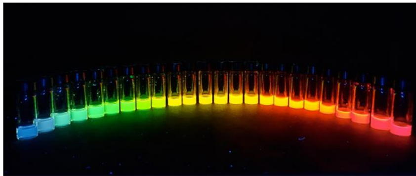
Figure 11: Image of quantum dots with different colors (due to their varying size and chemical composition).
