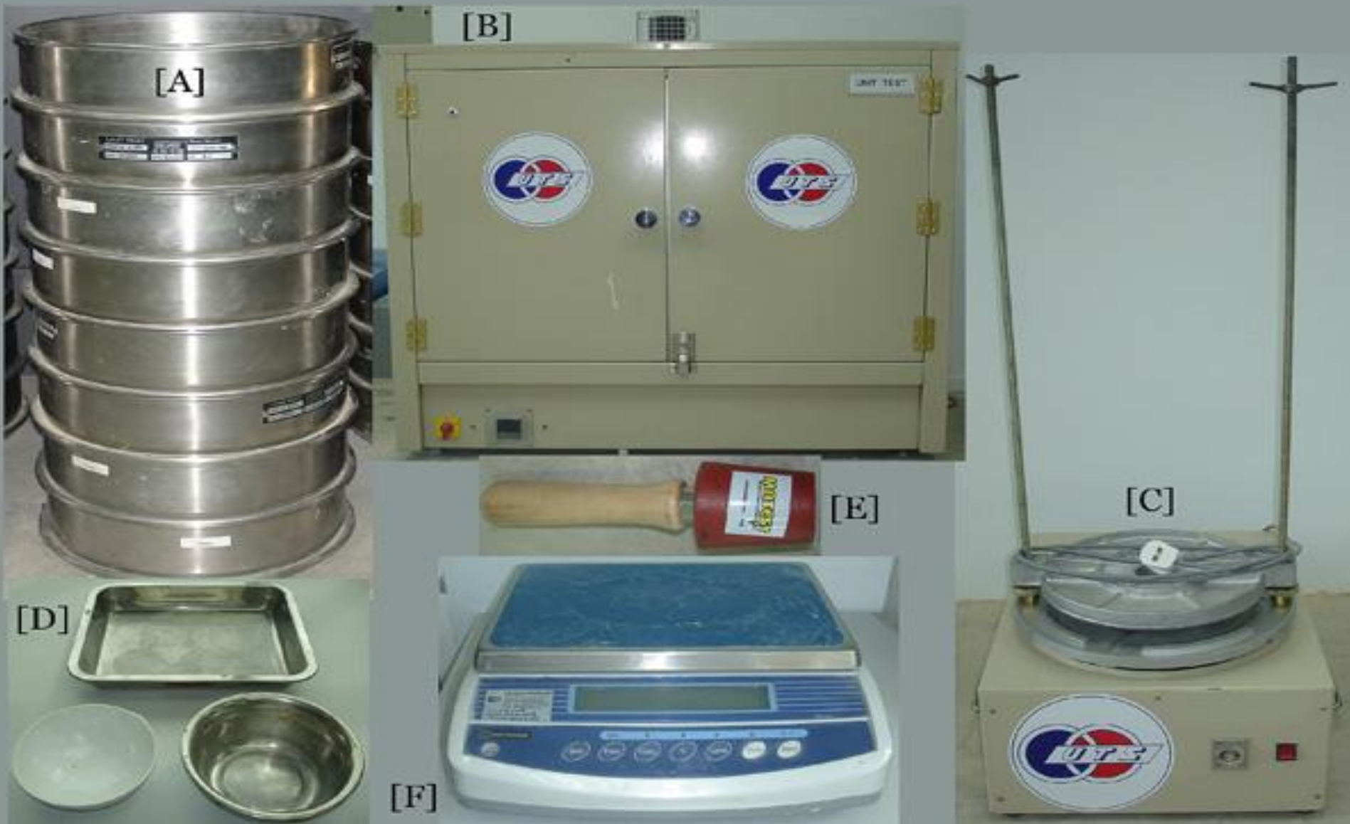
Sieve Analysis Apparatus: A) Sieve aperture sizes, B) Dry oven, C) Sieve shaker, D) Mortar & Tray, E) Rubber pestle, [F] Balance
