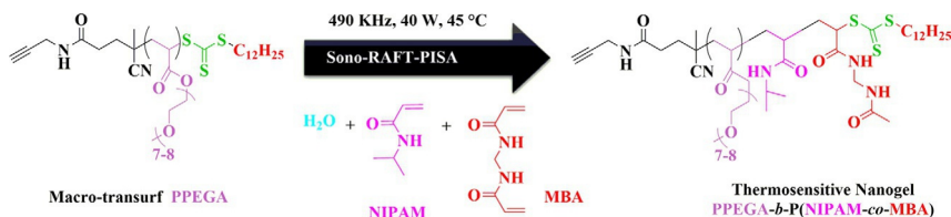
Scheme 7 Synthesis of thermosensitive nanogels-based on PPEGMA- b -P(NIPAM- co -MBA) [48].
