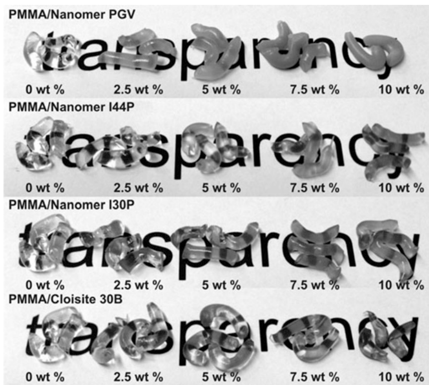
Fig. 10 Effect of nanoclay content on relative variation of opacity of PMMA/nanoclay nanocomposites [36]
