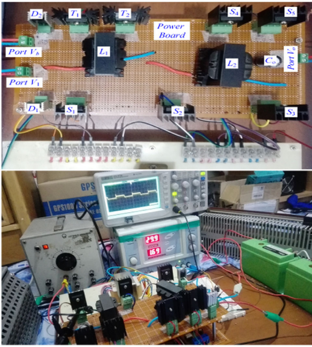
FIGURE 10 Laboratory image of the converter with experimental setup
