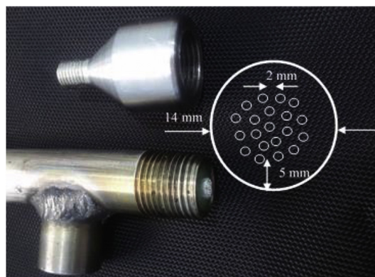
Fig. 1. Configuration of the air gap membrane distillation module.
