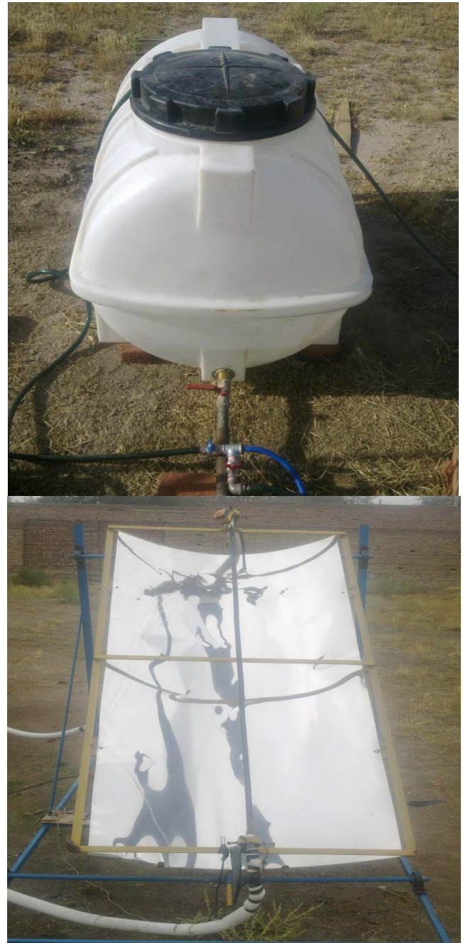
Fig 1. The schematic of solar dryer equipped with: chassis, reflector, receiver tube, thermal controller, centrifugal pump.
