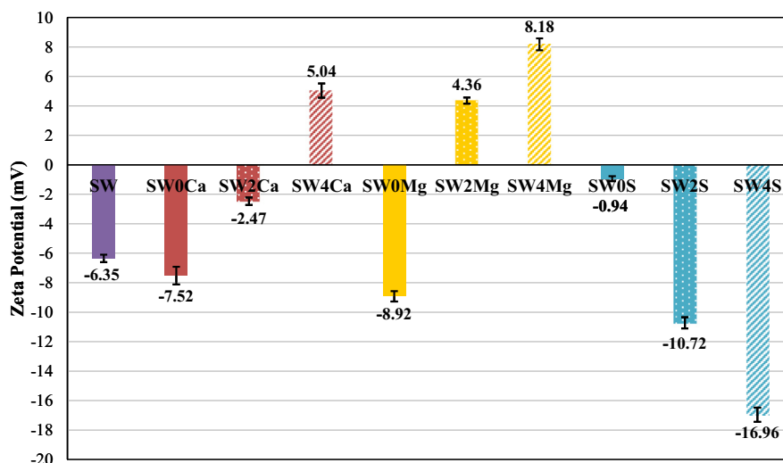
Fig. 4. Zeta potential of calcite fine particles aged in various brines including sea water (SW), and different divalent ions concentrations ( \text{Ca}^{2+} , \text{Mg}^{2+} and \text{SO}_4^{2-} ) at room temperature.
