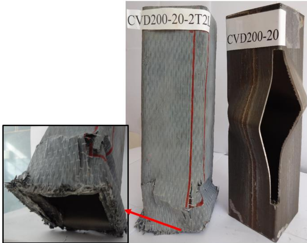
Fig. 11. Failure modes of the specimens with corner deficiency: non-strengthened and strengthened
