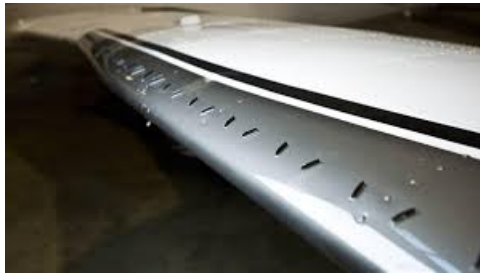
Figure 19: way of vortex generator resident
