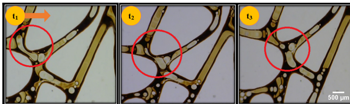
Fig. 16. Snap-off mechanism observed in the porous medium during the injection of \text{Al}_2\text{O}_3/\text{SiO}_2 CTAB foam (0.04 wt% \text{Al}_2\text{O}_3/\text{SiO}_2 NPs and 0.08 wt% CTAB). Subscripted numbers show the time passage.
