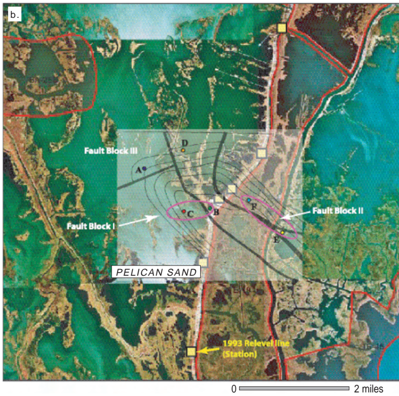
Figure 2.10. The Pelican sand of the Lapeyrouse field in southern Louisiana is highly compartmentalized. Note that in the early 1980s, while fault blocks I and III are highly depleted, fault block II is still at initial reservoir pressure (modified from Chan and Zoback 2006). Hence, the fault separating wells E and F from B and C is a sealing fault, separating compartments at pressures which differ by \sim 55 MPa whereas the fault between wells B and C is not a sealing fault.
