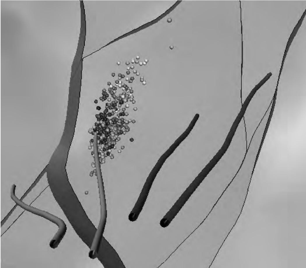
Figure 11.12. Perspective view of four wells in the Yufutsu gas field, some of the larger faults in the reservoir and the cloud of microseismicity induced by injection of 5000 \text{ m}^3 of water over 7 days (after Tezuka 2006). The cloud of seismicity is elongated along the direction of the vertical plane of a hydrofrac at the azimuth of S_{H_{\max}} .
