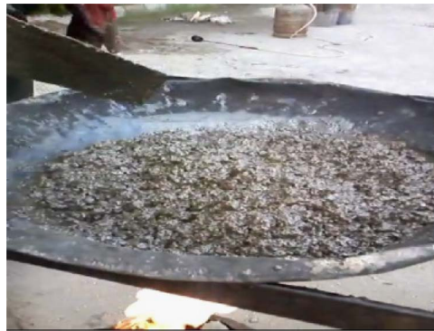
Fig. 8. Blending the sulfur cement and the heated aggregates and achieving the sulfur concrete.
