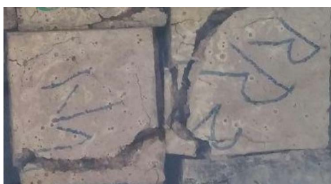
Fig. 1. Styrene modified concrete samples in water labeled 'Failed'.
